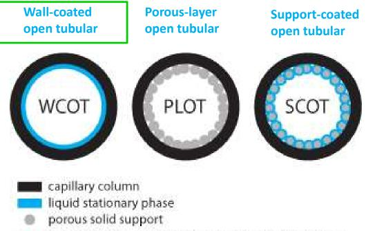
porous solid support coated w/liquid stationary phase
