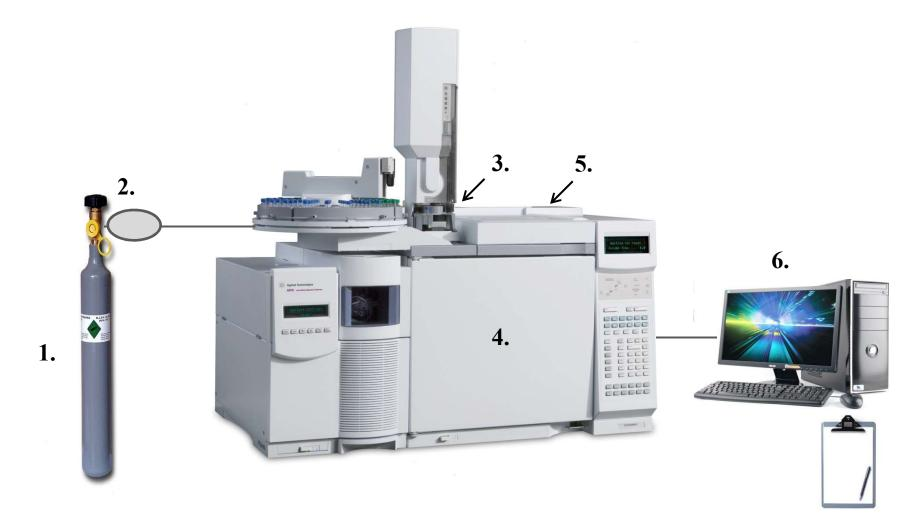
1: Mobile phase, 2: Pressure controller, 3: Injector, 4: Column, 5: Detector, 6: Data system
