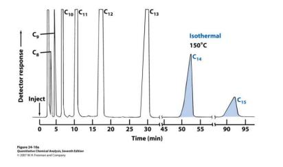
One difficulty with an isothermal separation is that the separation of a low-boiling solute may lead to an unacceptably long ret<u>ention time</u> and broad peaks for a higher-boiling solute.
