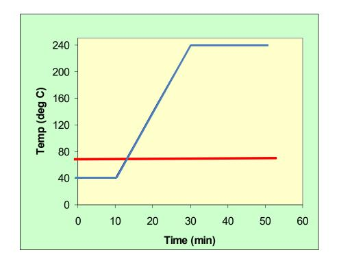
For **isothermal** operation (**red line**), the GC is held at a steady temperature during the analysis. In **temperature programmed** GC (**blue**) the oven temperature is increased according to a temperature program during the analysis.
