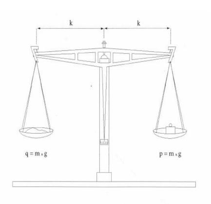
Equal-arm balance is the used most known, conventional, equal arm type weighting device, which can measure maximum 1000,0 g of materials, although its accuracy is 0,1g. **Quantities less than 1,0g** are not measured with this type of balance. In these cases latter mentioned scales can be used due to their accuracy.
