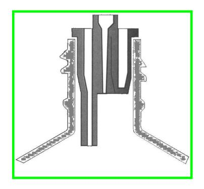
By manufacturer's preparations integral dropper is applied (central dropper adapter).
